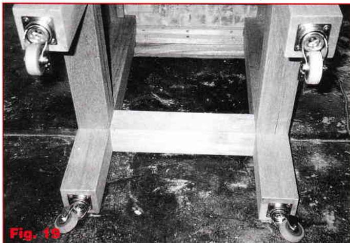
Chamfer the base of each leg slightly by hand sanding the edge at a 45° angle.
