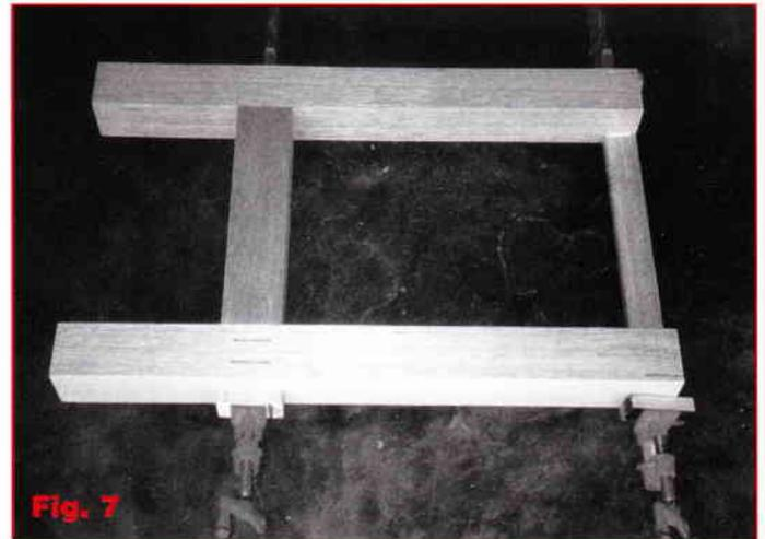
Check that everything is square by measuring the diagonals. Adjust the clamps until both measurements are identical.
