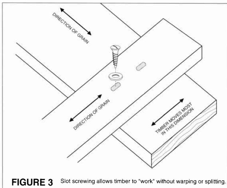
**FIGURE 3** Slot screwing allows timber to "work" without warping or splitting.
