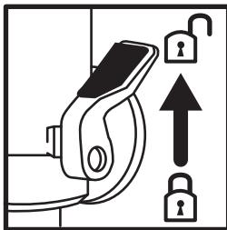
**Note:** To lock the router at a particular depth of cut, plunge the router head down and rotate the Plunge Lock Lever (18) to its lower position. This will hold the router head in this position.
