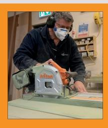
"After reading good reviews of this track saw, I decided to purchase one, and I wasn't disappointed. The saw gives a nice cut on veneer plywood, especially when using the scoring cut feature before making the through cut... For the money, this saw is excellent value.'
